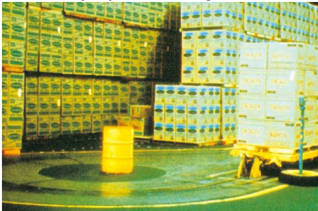
Towline conveyor system for stocking
