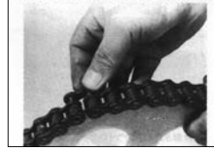
Chain clip installation method
